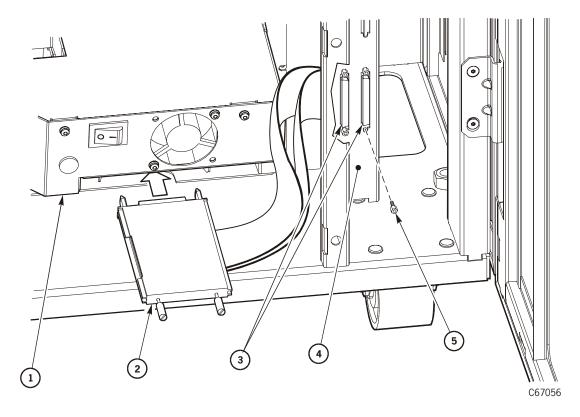
DLT Drive Cable Connections (C67056)
