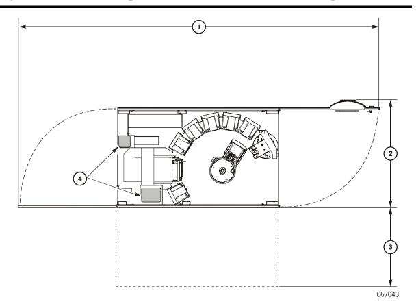
Figure 2-1. Service Area Requirements and Cable Access Locations (Top View)
