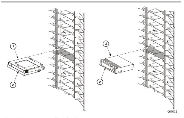
Placing Tapes into Array Cells (C67072)
