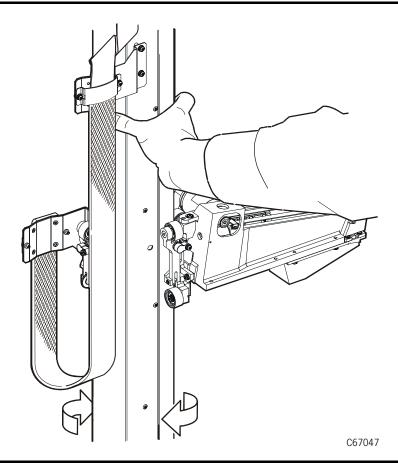
7. Raise the hand-camera assembly (on the Z carriage) as shown in Figure 2-7 so that you have comfortable access to the hand assembly. Remove and discard the foam packing material from inside the hand assembly.
