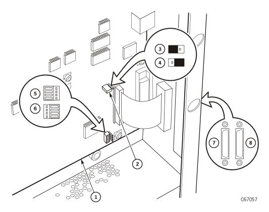
Terminating Power & Channel Setting Jumpers—L180 (C67057)
