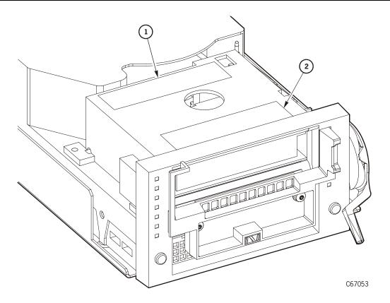
DLT Model Number and Operation Type Labels (C67053)
