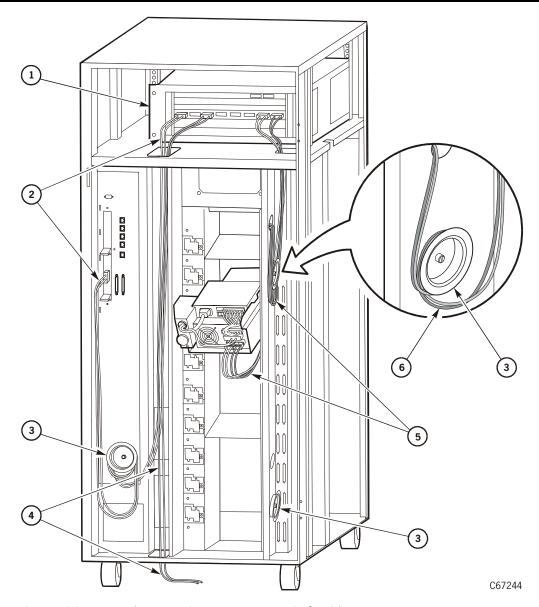
L180 Fiber Cable Route from Rack Area to Drive (C67244)
