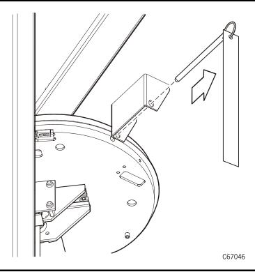
5. Retain the shipping pins. They are required for maintenance procedures to the Z and theta motors. Pins may be stored in holes provided in the rack floor. These holes are located in the front on the right-hand side.
