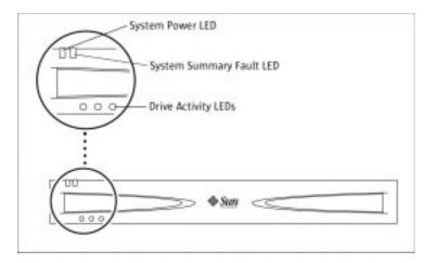
Figure 3. Front Panel System Power/Fault Indicators
