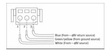
Figure 9. DC input power cables
