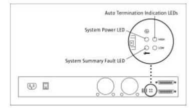
Figure 7. Rear Panel LEDs
