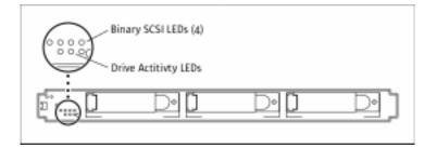
Figure 4. Front Panel Disk Drive LEDs
