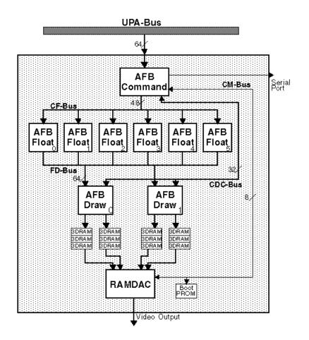
Figure 3. Sun Elite3D m6 graphics chip-level diagram
