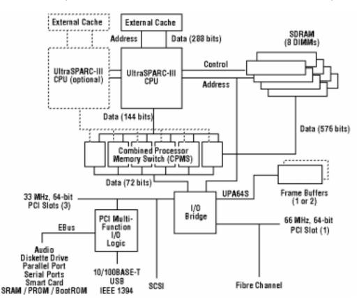
Figure 2. Architecture of the Sun Blade 1000 and 2000 system
