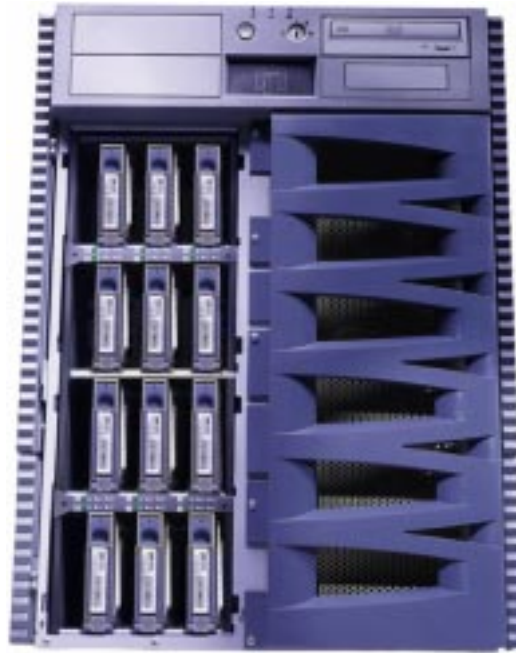
Figure : Sun Fire™ V880 Server, front view 12 FC-AL disk drives
